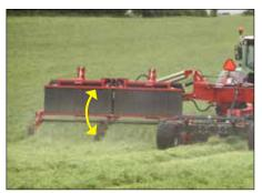
Collector is not activated and the GXT can then make wide spreading.
