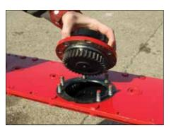
The Top Service design of the cutter bar makes it possible to check and replace a gear wheel or bearing on each disc
