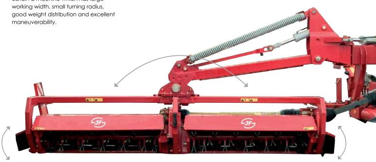
All GXT-machines have pendulum suspension which ensures that the already low ground pressure is distributed evenly over the whole width of the cutting unit which spares the grass roots. You obtain optimal ground adaptation and strong lateral forces on the tractor are avoided.
