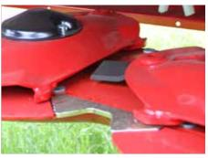
The counter knife is 2 mm higher than the cover of the cutter bar
