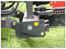
Top safe ensures low impact on the cutter bar while driving with high speed.
