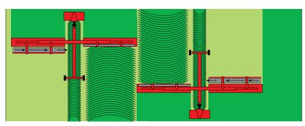
One big wide-spread swath from a working width of 24 m, which can be raked into one swath.
