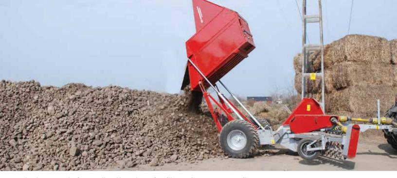
The hopper design on the Stonebear is with a 1.8 cu. m capacity.
