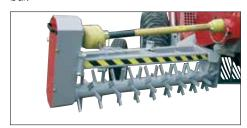
The Stone rake collects the stones to the drum.
