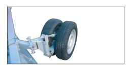
Adjustable double wheels control the depth of the SB 5200 stone rakes.
