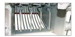
The collecting drum of SB4000 has a rotor with 18 and SB5200 24 Kongskilde tines.
