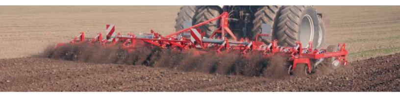
Kongskilde Vibro Master 3000 is a fully-mounted seedbed cultivator equipped with vibrating tines in working widths from 21' to 27', for tractors up to 250 hp.
