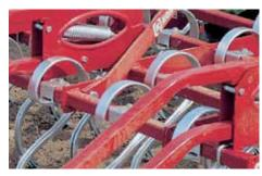
Oval Beam-Truss frame design for added strength.
