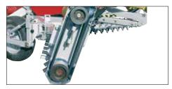
A V-belt pulley powers the stone rakes.
