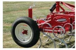
Crank Adjustment Gauge Wheel
