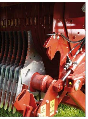
Sharp knives at any time - Thanks to the patented quick release system
