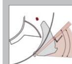
Spring tension holds the knife in the duct even in the event of the knife coming into contact with a foreign object. As a result of the constant spring tension, the knife blade becomes blunt due to the greater force acting on the blade through the foreign object.
