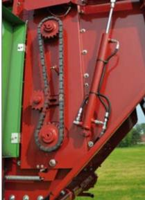
• Driven by large-sized roller chains • Safety switch-off at the bottom beater
