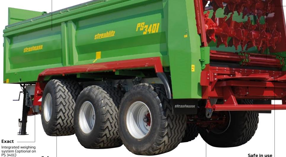
Hydraulic chassis with lift axle for steady roadability
